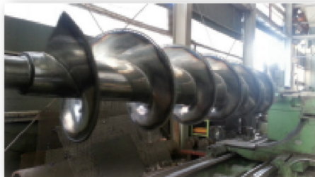
MAIN SCREW FABRICATION
